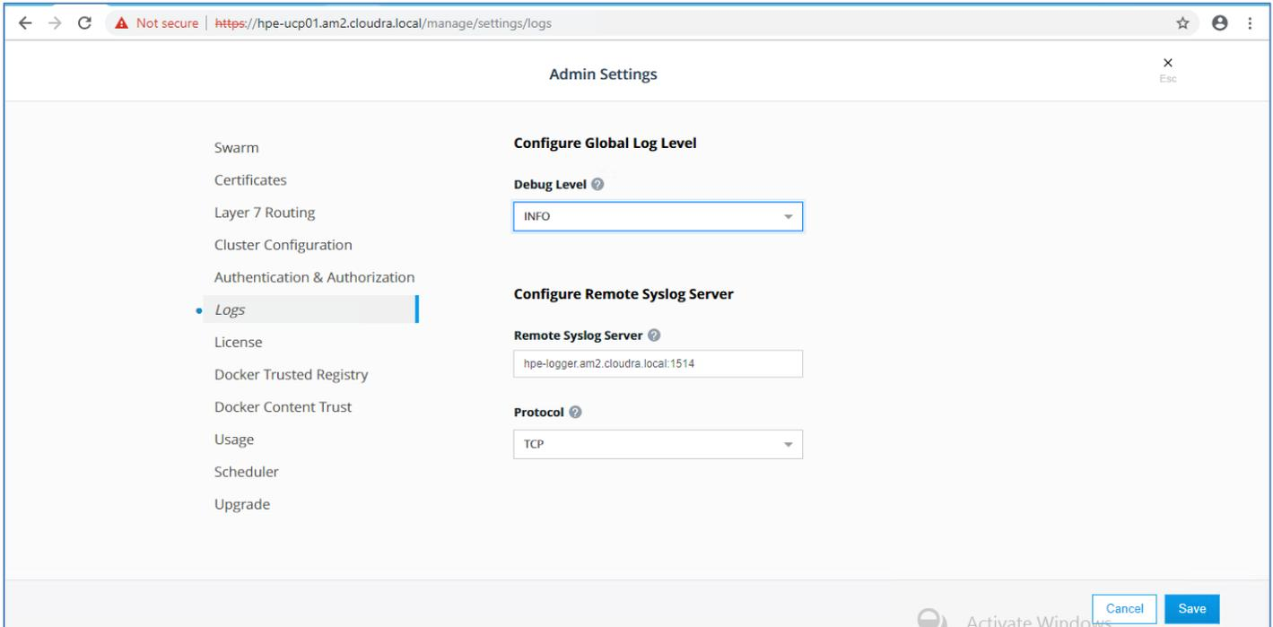
Figure 23. Configure Remote Syslog Server in UCP
